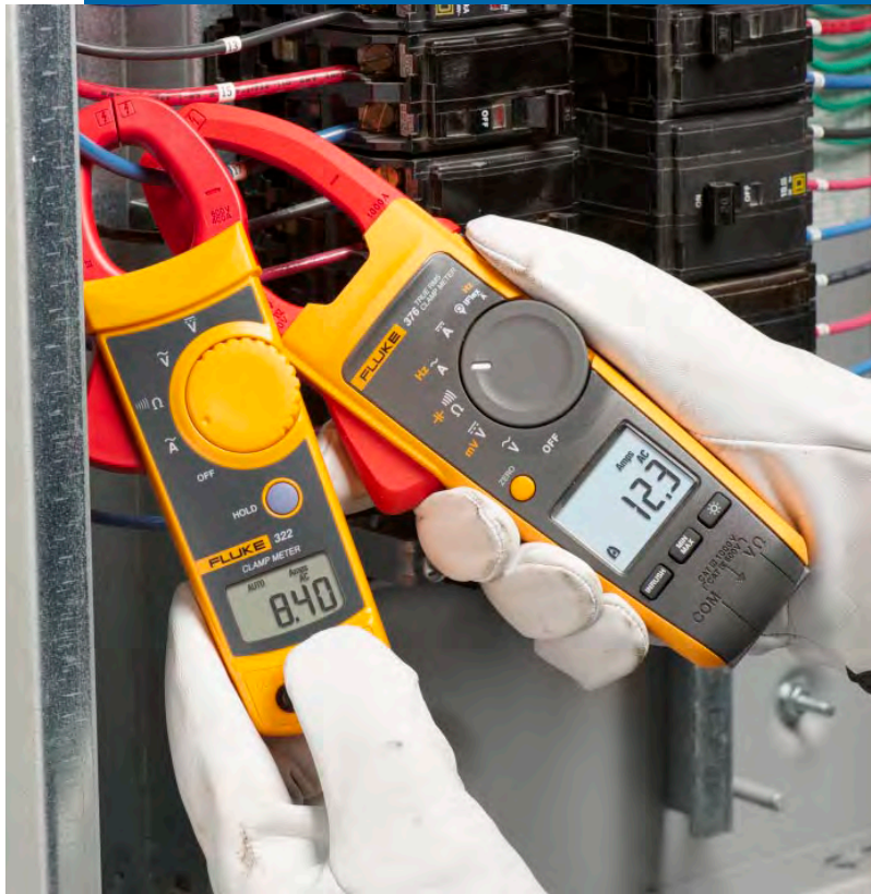
One current—two readings. Which do you trust? The branch circuit above feeds a non-linear load with distorted current. The true-rms clamp reads correctly but the average responding clamp reads low by 32 percent.
