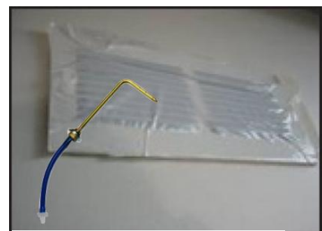
Figure 17: A Static Pressure Probe attached to a pressure tube allows the measurement of pressure without flow interference (e.g.: inside a supply
