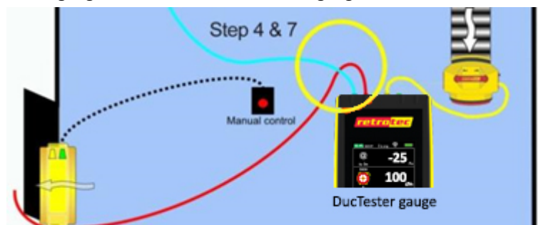
Figure 33: 1 Gauge Duct Leakage to Outdoors under depressurization, setting the duct pressure
