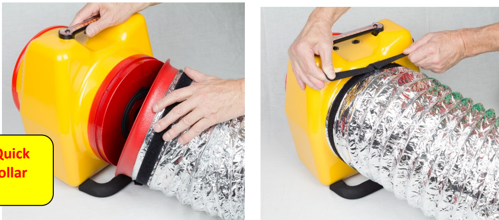
Figure 22: Install Flex Duct over the fan inlet, covering the Range Rings, for depressurization. Tighten the strap.
