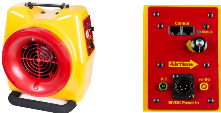
Figure 4: Retrotec Model 300 has a speed control knob and two Ethernet style Speed Control Ports for daisy chaining speed controls for running many fans together. The yellow and green color coded tubing connections to the gauge are shown.
