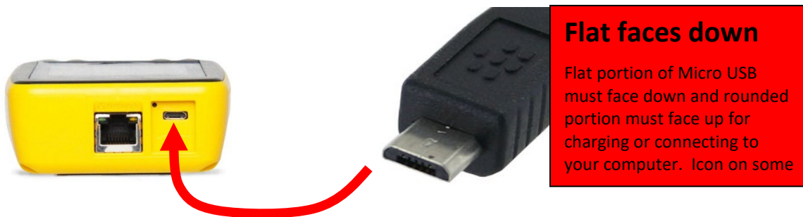
Figure 14: Electrical connections on the bottom of the gauge include Network (Ethernet) Cable that goes from the DM32 to a PC (if Retrotec PC software is used for data collection), micro USB cable for PC software and/or charging, and a reset button.
