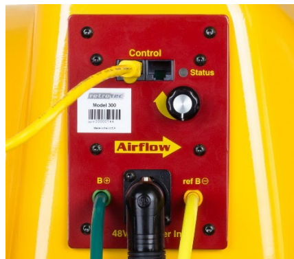
Figure 15: Model 300 Fan Top houses the speed control, control knob, power connection, color-coded tubing connections (green and yellow) and Control Cable.
