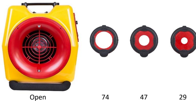
Figure 3: Open Range is for the leakiest ducts and houses while Ranges 74, 47, 29 are for progressively tighter ducts.
