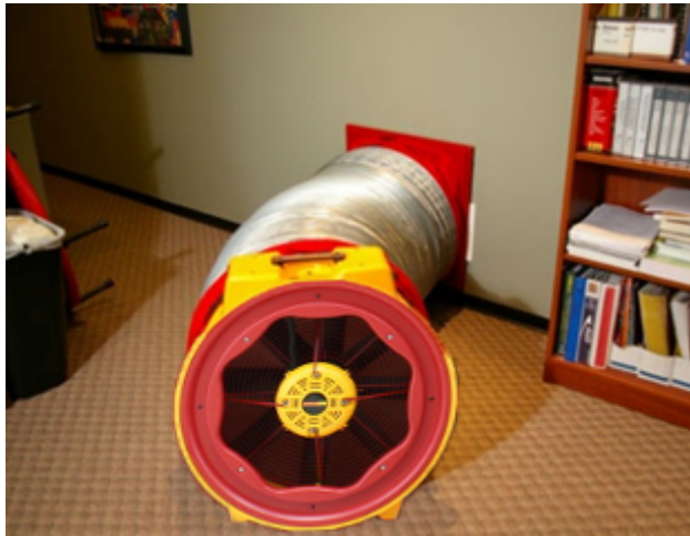
Figure 41 Flex attached to Blower Door
