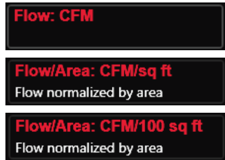
Figure 24: Some of the most common results that can be read directly off the gauge.
