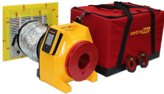
Figure 2: A complete duct testing system.
