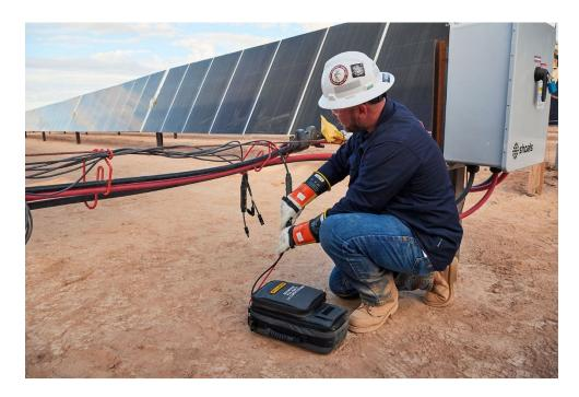
The Fluke Solmetric PVA-1500 is a cutting-edge I-V curve analyzer kit designed to ensure accurate energy measurement and optimal system function. With this high-precision testing equipment, you can reliably assess the health and efficiency of your solar modules, making informed decisions to enhance their output and longevity.
