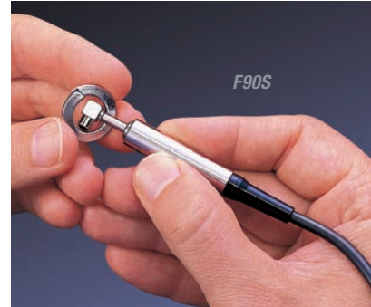
Microprobe series for small parts and hard-to-reach areas
