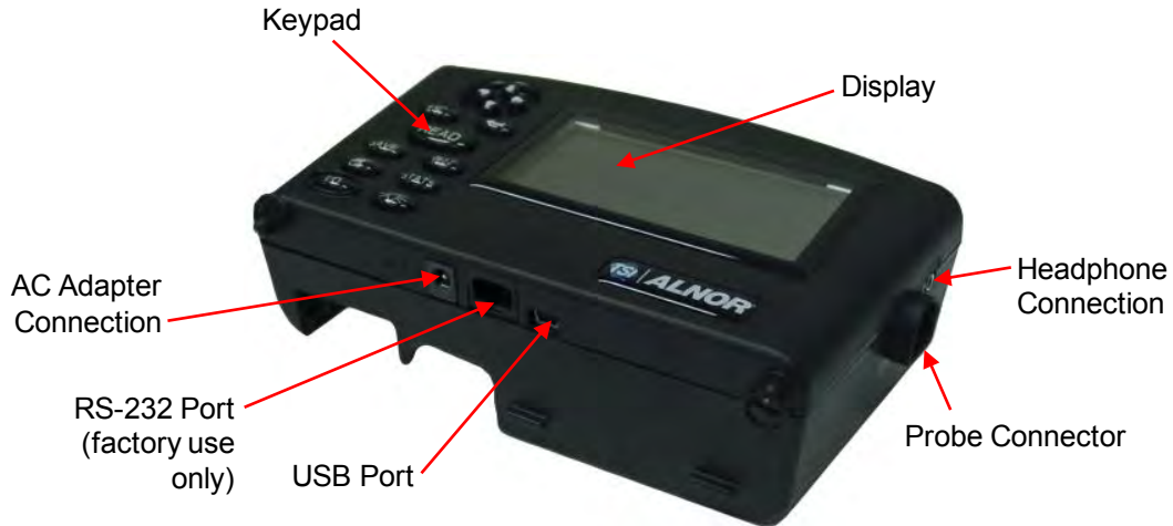
Figure 1: Features of the EBT730/EBT731 Micromanometer, Front View
