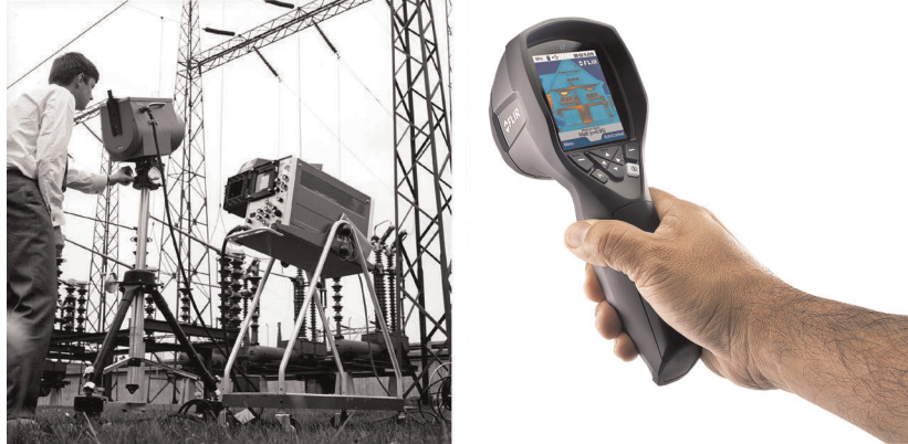
Figure 12.2 LEFT: Thermovision Model 661 from 1969. The camera weighed approximately 25 kg (55 lb.), the oscilloscope 20 kg (44 lb.), and the tripod 15 kg (33 lb.). The operator also needed a 220 VAC generator set, and a 10 L (2.6 US gallon) jar with liquid nitrogen. To the left of the oscilloscope the Polaroid attachment (6 kg/13 lb.) can be seen. RIGHT: FLIR i7 from 2012. Weight: 0.34 kg (0.75 lb.), including the battery.
