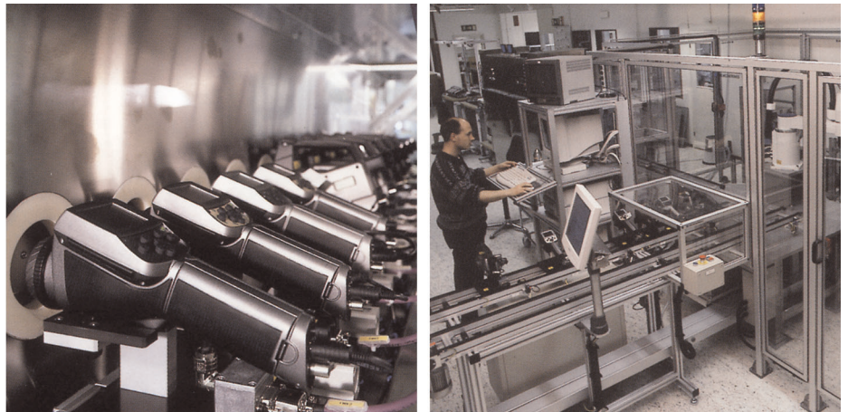
Figure 12.5 LEFT: Testing of infrared cameras in the climatic chamber; RIGHT: Robot used for camera testing and calibration
