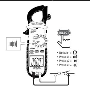
$\bullet$  Buzzer sounds at less than 40  $\!\Omega.$
