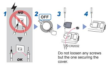
Do not turn any one of the three screws inside the battery case. Doing so will cause the instrument to report abnormal measured values.
