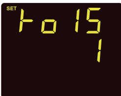
Fig 3-28 RO1 Alarm Inequality Setting
