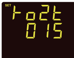
Fig 3-36 RO2 Alarm Delay Setting
