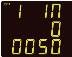
Fig 3-2 Full range current setting
