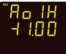
Fig 3-21 AO1 Up Limit Setting
