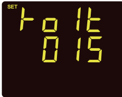
Fig 3-30 RO1 Alarm Delay Setting
