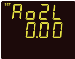
Fig 3-23 AO2 Lower Limit Setting
