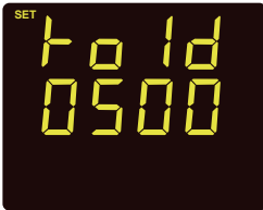
Fig 3-26 RO1 Momentary Delay Time
