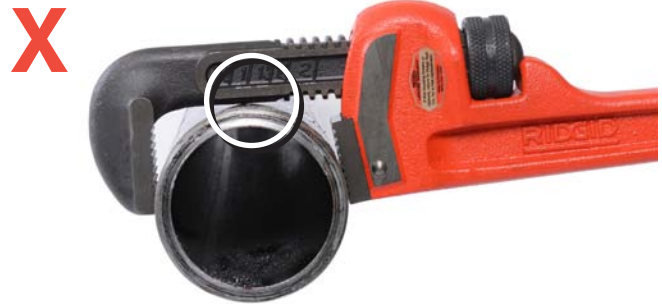
Figure 4 – Wrench Too Small For Work Piece, Hook Shank Touching Work Piece.
