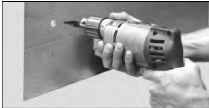
1. Drill 1/2" pilot hole using Greenlee Kwik-Stepper® step bit.
