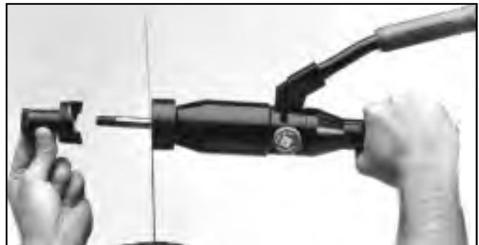
5. Thread the adapter with punch onto the draw stud as shown.
