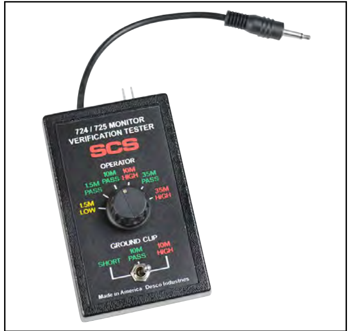
Figure 12. SCS 770065 Verification Tester
