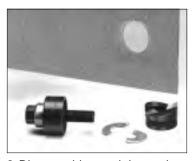
8 Disassemble punch by turning draw stud counter-clockwise while holding punch. Tip die and drop out split slugs.
