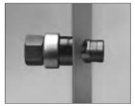
3 Thread punch on draw stud with cutting edge toward material being punched.
