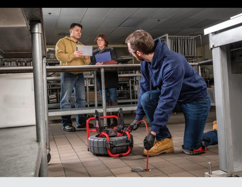
The RIDGID® SeeSnake® CSx Via is a flexible, bring-your-own-screen solution, providing a convenient means to stream, capture, and share superior inspection images using an iOS, Android, or Windows device. The CSx Via utilizes the free HQx® Live app to remotely control the camera functions and features, such as the distance counter and the sonde. CSx Via is also compatible with TruSense® SeeSnake systems and will enable TruSense features in the app.
