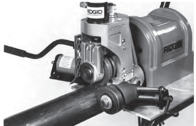
Figure 10 – Adjusting Pipe Stabilizer
