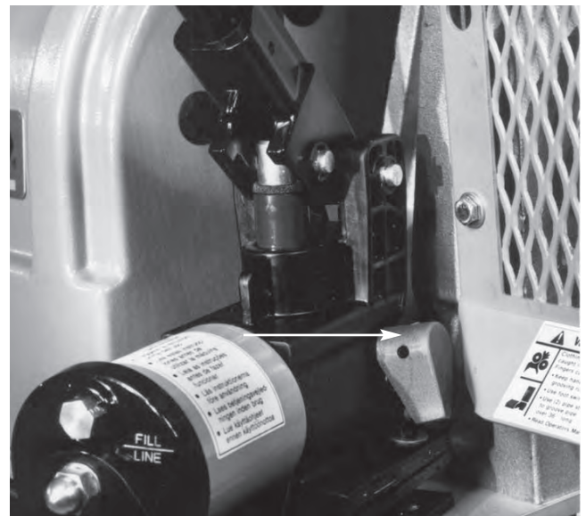
Figure 4 – Close-up of Release Lever on 918-I Pump
