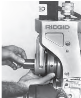
Figure 12 – Remove Groove Roll Shaft and Groove Roll
