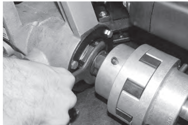
Figure 14 – Loosen and Remove Drive Shaft Retaining Nut
