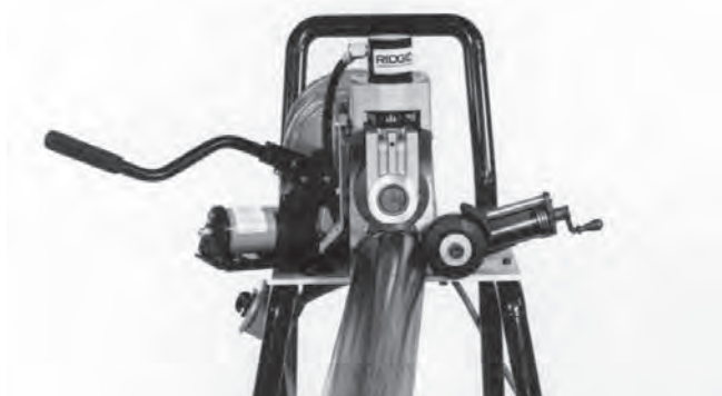
Figure 7 – Offset Pipe on 918-I (exaggerated for clarity)
