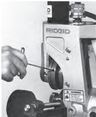
Figure 11 – Loosen Set Screw in Groove Roll
