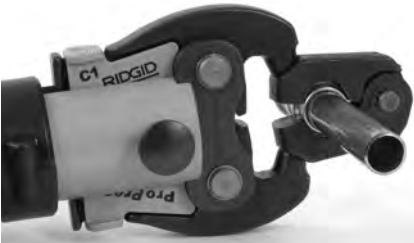
Figure 10 – Attaching Actuator to Press Ring
