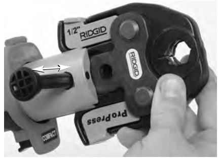
Figure 6 – Attachment Mounting Pin
