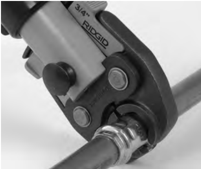
Figure 7 – Placing Scissor-Style Jaws Around Fitting
