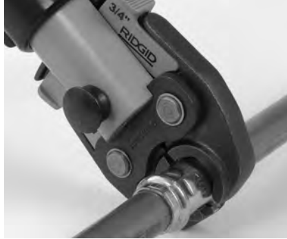
Figure 7 – Placing Scissor-Style Jaws Around Fitting
