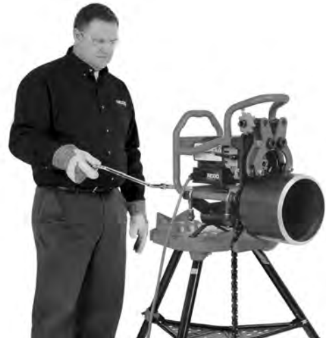
Figure 20C – Bevelling Operation (Fixed Beveller/Rotating Pipe)
