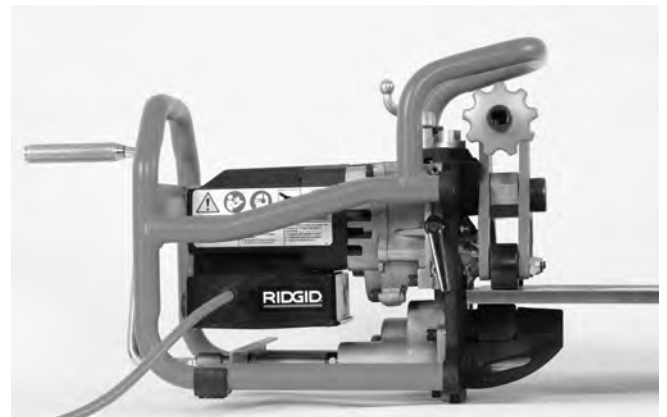
Figure 16B – Installing Beveller on Plate
