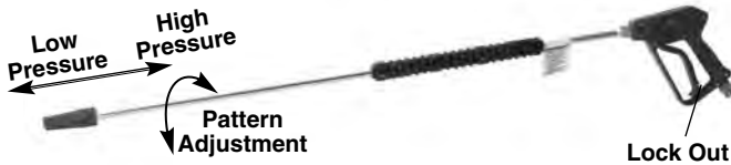
Figure 17 – Wash Wand Nozzle Adjustments
