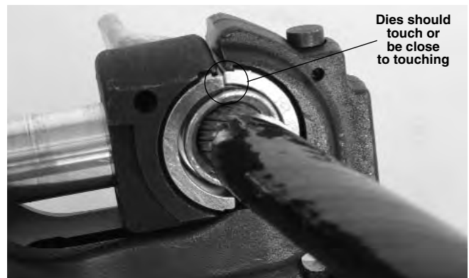
Figure 8 – Inspecting Dies as Pressure Relief Valve activates
