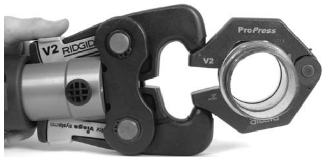
Figure 9 – Attaching Actuator to Press Ring
