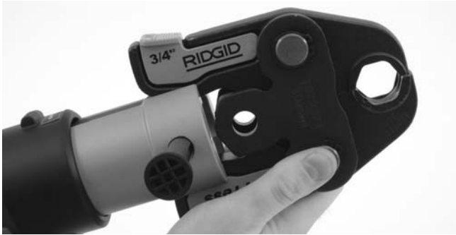
Figure 5 – Slide Attachment Into Tool
