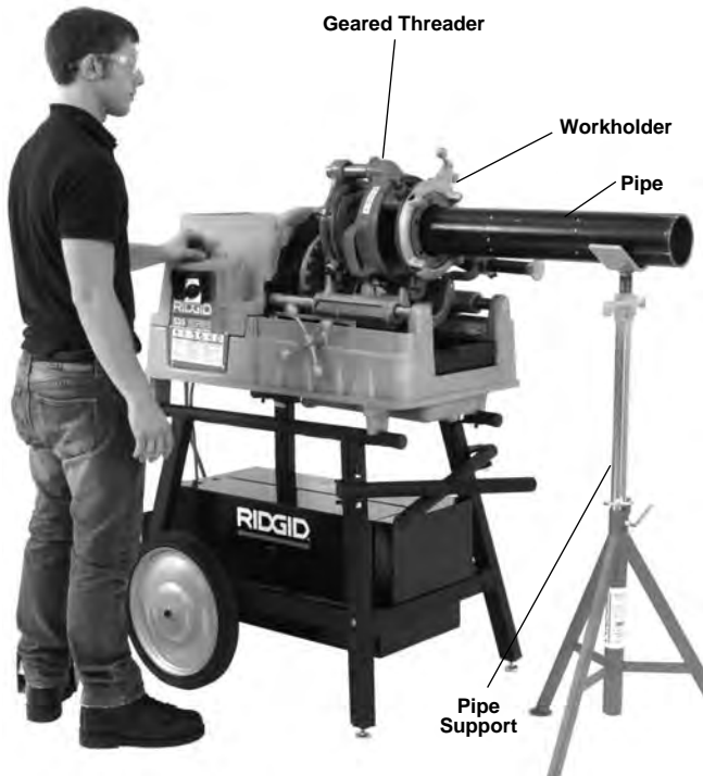
Figure 21 – Operating Position (Close-Coupled Method)
