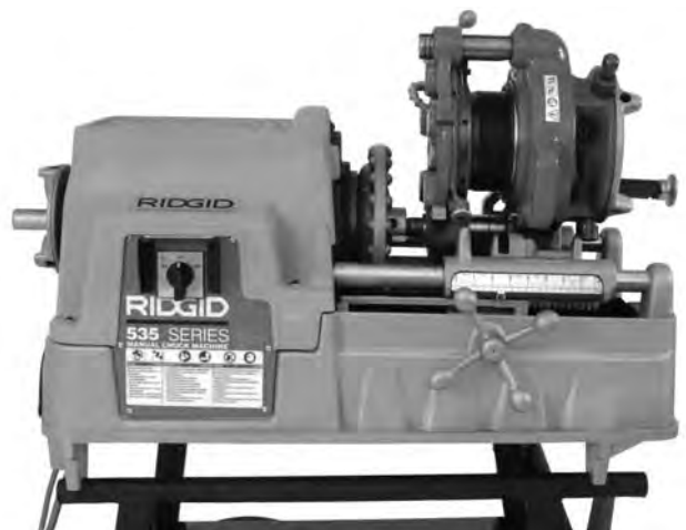
Figure 17 – Geared Threader Close-Coupled To 535
