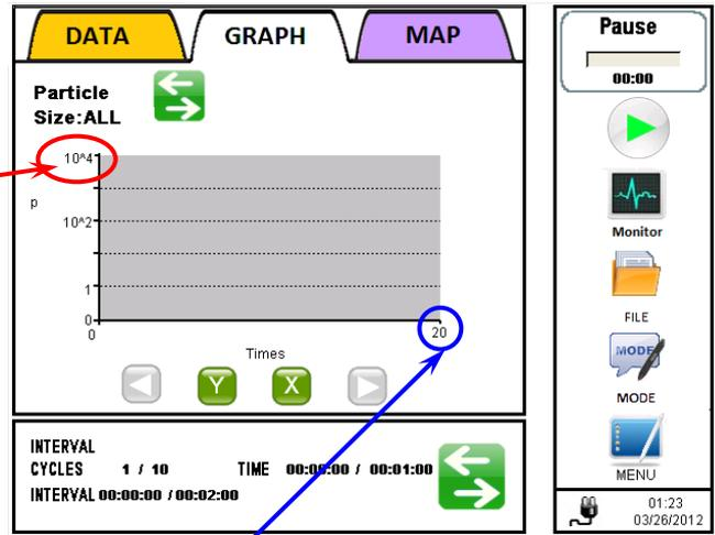
**X Axis: MAX value** set in the PARTICLE tab in the CHART SETTING window is applied to the chart.
