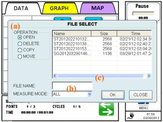
Select [FILE] on the initial screen. Then a screen shown to the left will be displayed. You can display, print and delete data here. You can also display the list of files that has been outputted in the ALARM/ERROR LOG screen.
