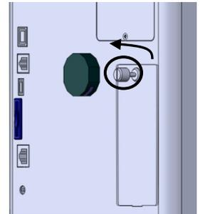
Open the battery compartment cover on the rear of the instrument.
