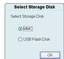
**\*After files are moved to the MMC card or USB flash drive, they are deleted from the internal data storage.**
