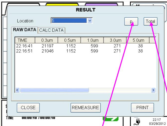
When all of the measurements are finished, a final measurement result will be displayed.
