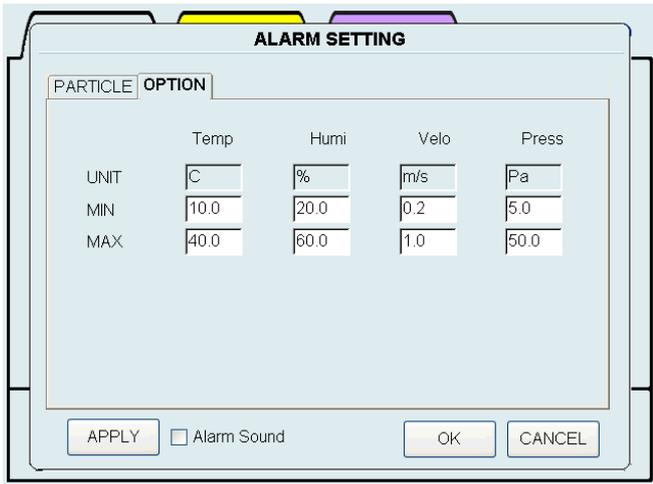
In the OPTION tab, you can set an alarm threshold for TEMPERATURE, HUMIDITY, VELOCITY and DIFFERENTIAL PRESSURE.
