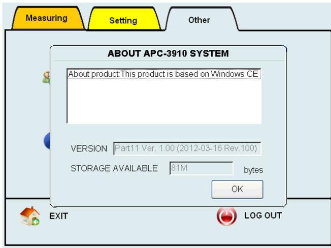
Tap [ABOUT] to view the firmware version of the instrument and the remaining capacity of the internal data storage.
