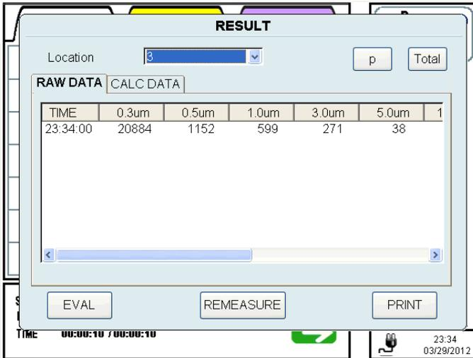
When all measurements are finished, the final measurement results will be displayed. You can view the result of a certain LOCATION POINT by selecting Location from the dropdown list.
