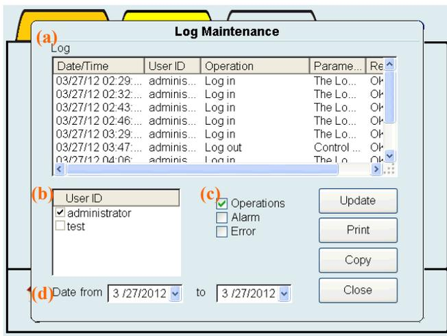
The "Log Maintenance" screen shows up when you select "LOGS" on the control panel. Users can review and print-out the log files, such as the operation log, alarm log, and error log
