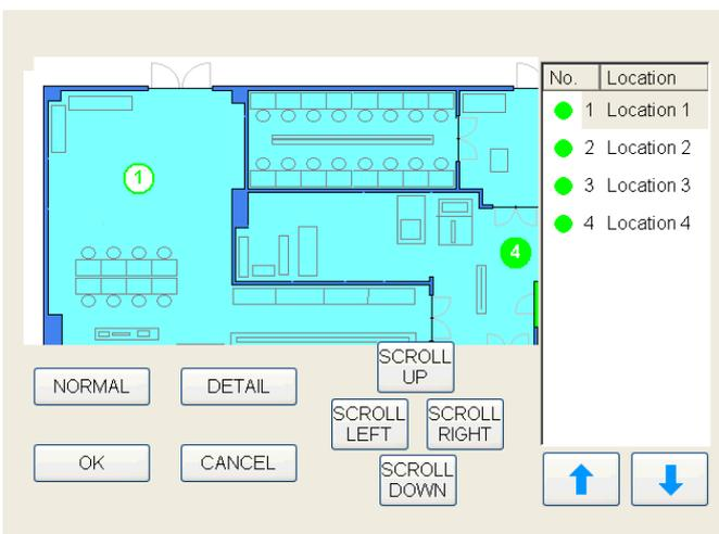
When a MAP is enlarged, [SCROLL UP], [SCROLL DOWN], [SCROLL LEFT] and [SCROLL RIGHT] buttons are activated, which enables you to move the MAP.
