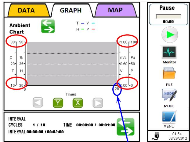
The **MAX and MIN values** set for each sensor in the OPTION tab in the CHART SETTING window is applied in the chart.
