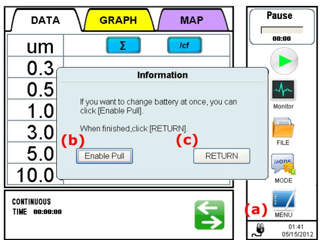
If you must exchange the battery when the power is on and the battery is charging, you can follow this instruction:
