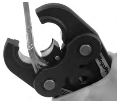
Figure 13 – Cleaning Segment Area of MegaPress Jaw
