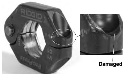
Figure 11 – Damaged Ring Pocket
