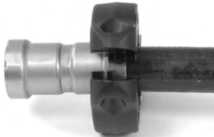
Figure 10 – Opening the MegaPress Ring and Placing Around Fitting
