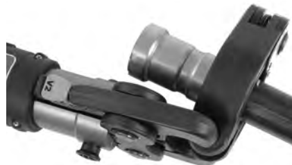
Figure 12B – Placing Actuator Into MegaPress Ring Pockets At An Angle For Additional Clearance
