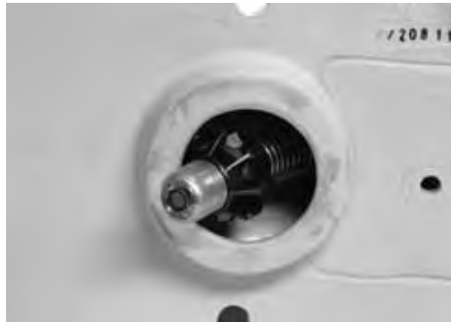
Figure 21 – Camera Head with Ball Guide in Turn
