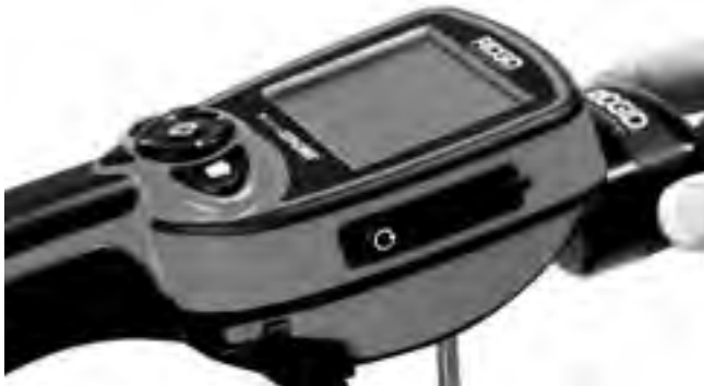
Figure 10 – Connecting the microEXPLORER Camera Monitor
