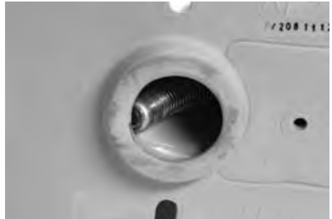
Figure 20 – Camera Head Blocked in Turn
