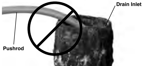
Figure 18 – Avoid Pulling At Sharp Angles
