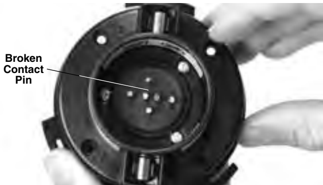
Figure 7 – Broken Contact Pin
