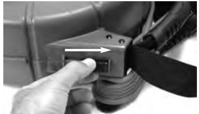
Figure 4 – Unlatching the microDrain Reel Case
