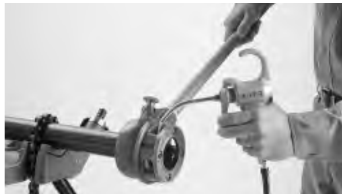
Figure 4 – Applying Thread Cutter Oil
