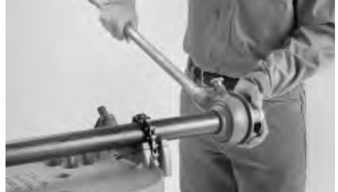
Figure 3 – Sliding Threader On Pipe
