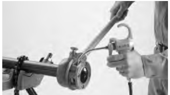
Figure 4 – Applying Thread Cutter Oil
