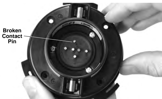
Figure 12 – Broken Contact Pin
