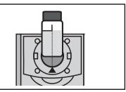
6. Remove tube from colorimeter. Add 5 drops of DPD 1A Free Chlorine Reagent (P-6740) and add 5 drops of \*DPD 1B Free Chlorine Reagent (P-6741), Cap and invert to mix. The solution will be pink if chlorine is present. Read within 30 seconds.
