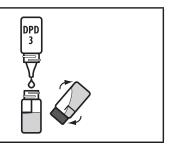
NOTE: For wastewater samples, <u>Standard Methods for the Examination of Water and Wastewater</u> recommends waiting 2 minutes for full color development when testing total chlorine.
