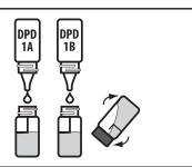
7. Immediately insert tube into chamber. Close lid. Select **Scan Sample**.
