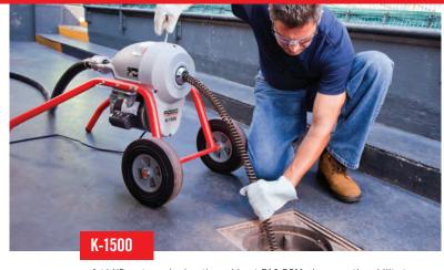
A % HP motor spinning the cable at 710 RPM gives you the ability to clean larger lines for longer distances and cut through blockages FAST!
