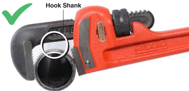
Figure 3 – Maintain Gap Between Hook Shank and Work Piece
