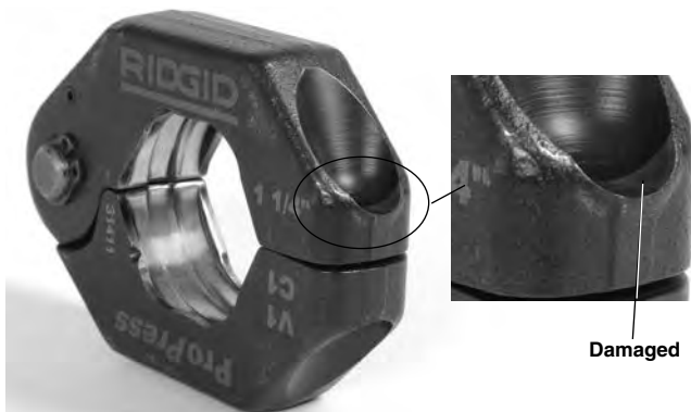
Figure 13 – Damaged Ring Pocket
