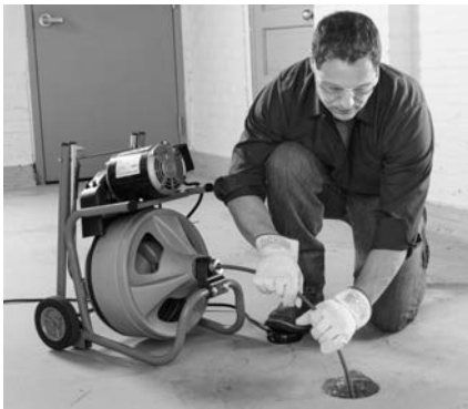
Figure 13 – In Operating Position, Manually Feeding Cable
