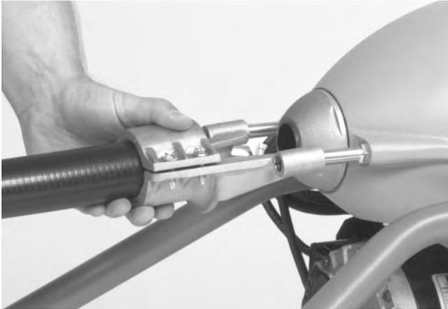
Figure 3 – Rear Guide Hose Attachment
