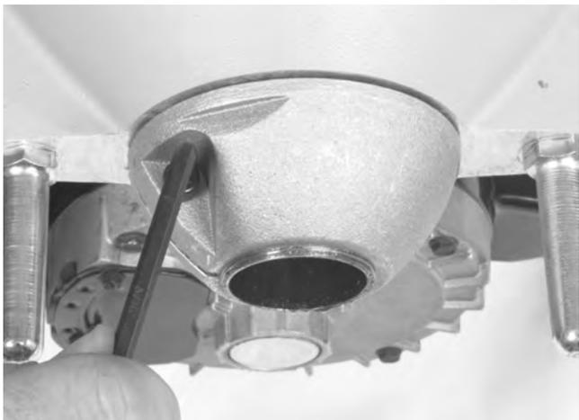
**Figure 14 – Removing Clutch End Play**
