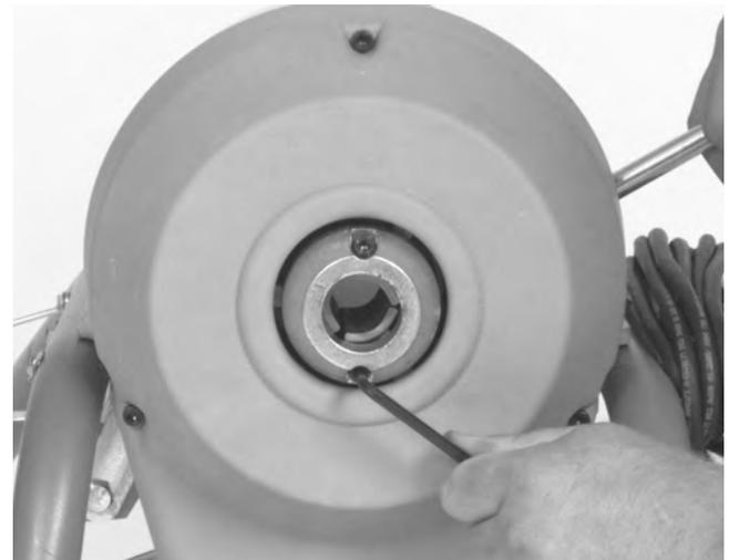
Figure 12 – Replacing Clutch Jaws
