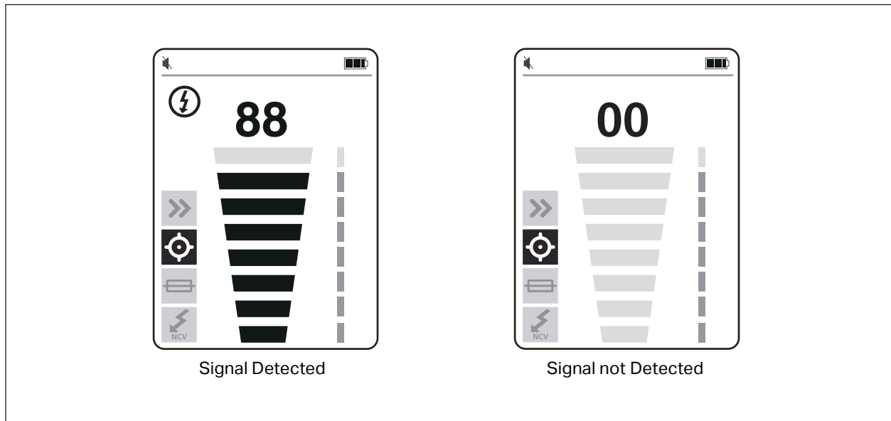
Figure 10. Tip Sensor Signal Strength (2052R)
