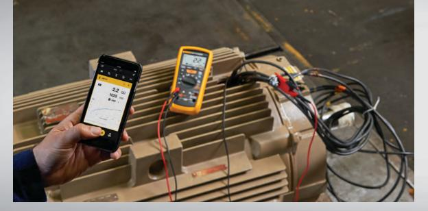
A digital insulation tester and full-featured multimeter—TWO TOOLS IN ONE!
