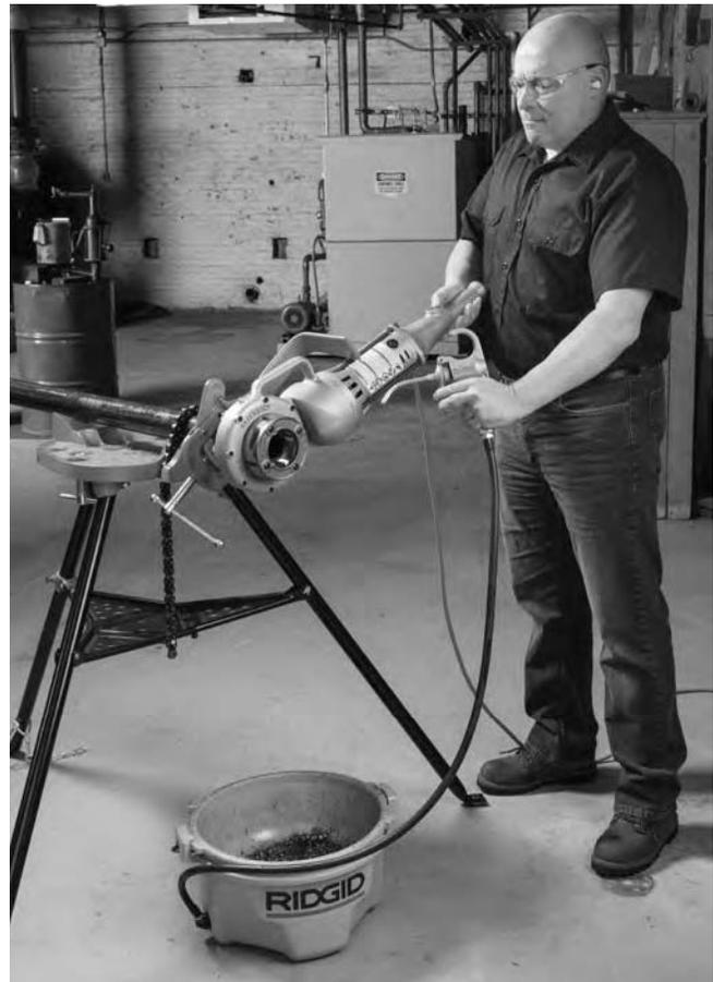
**Figure 9 – Threading Pipe**
