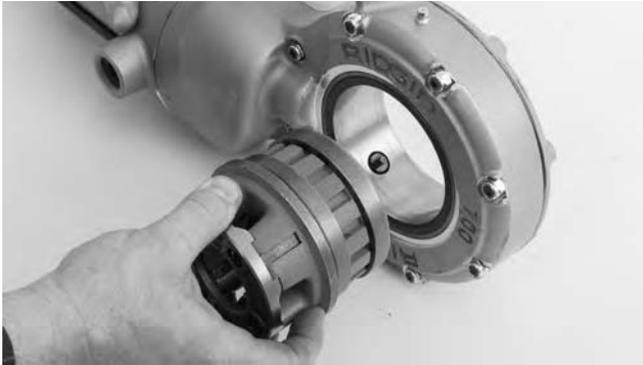
Figure 4 – Installing Die Heads into 700 Power Drive
