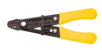
Klein Tools 1004 Wire Stripper and Cutter is a handy, light, compact tool for stripping insulation. Spring-loaded for action for self-opening. Convenient hole for looping or bending wire. Adjustable slide stop with set screw for repeat stripping work.
