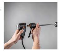
2 Fit new probe module and click into place.
