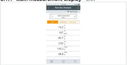
The measurement units and the number and order of the measurement parameters displayed in the Main measurement display – List, can be changed, see section Configure measurement display.
