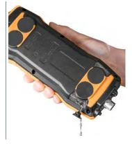
3 - Wipe off any drops still on the condensate outlet with a cloth and close the condensate outlet.
