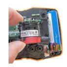
Remove hose connections from the faulty sensor/bridge.
