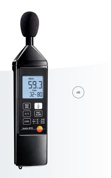
The testo 815 is the ideal instrument for the evaluation of sound level in everyday work. The instrument can be used for monitoring measurements in the areas of air conditioning or heating, on combustion plants or at workplaces, however machine or discotheque noise can also be evaluated quickly and precisely.
