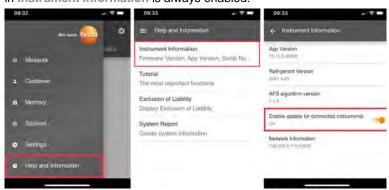
If a new firmware is available for your measurement instrument, an update notification is shown after connecting the instrument with the testo Smart App.
