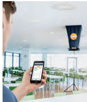
Testo 420 Bluetooth App allows for Smart, hands-free operation. Display and create custom reports on mobile devices. Send reports via email from the job site.
